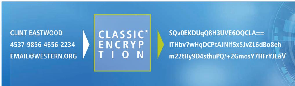
*\*Algorithm: Des; Mode: CBC; Output encoded using Base64*
